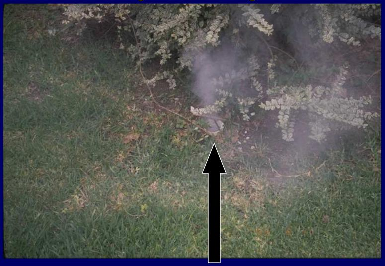
Most typical defect discovered - missing cleanout cap - easily remedied, but often removed again to provide yard drainage
